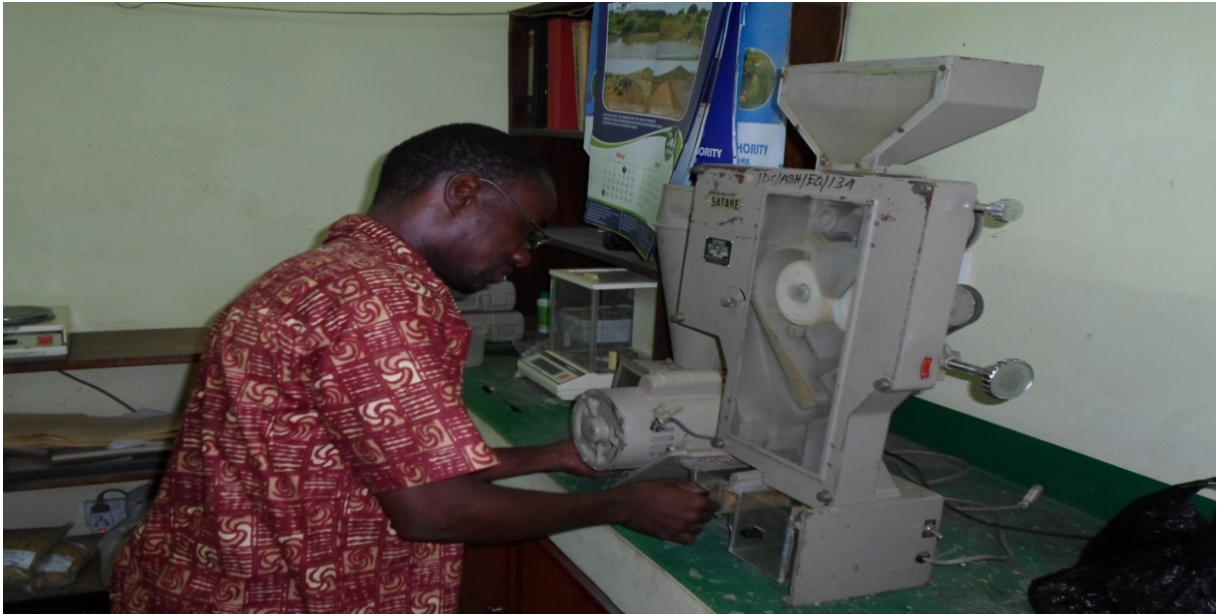
Plate 3: Experimental machine used to mill the rice samples
