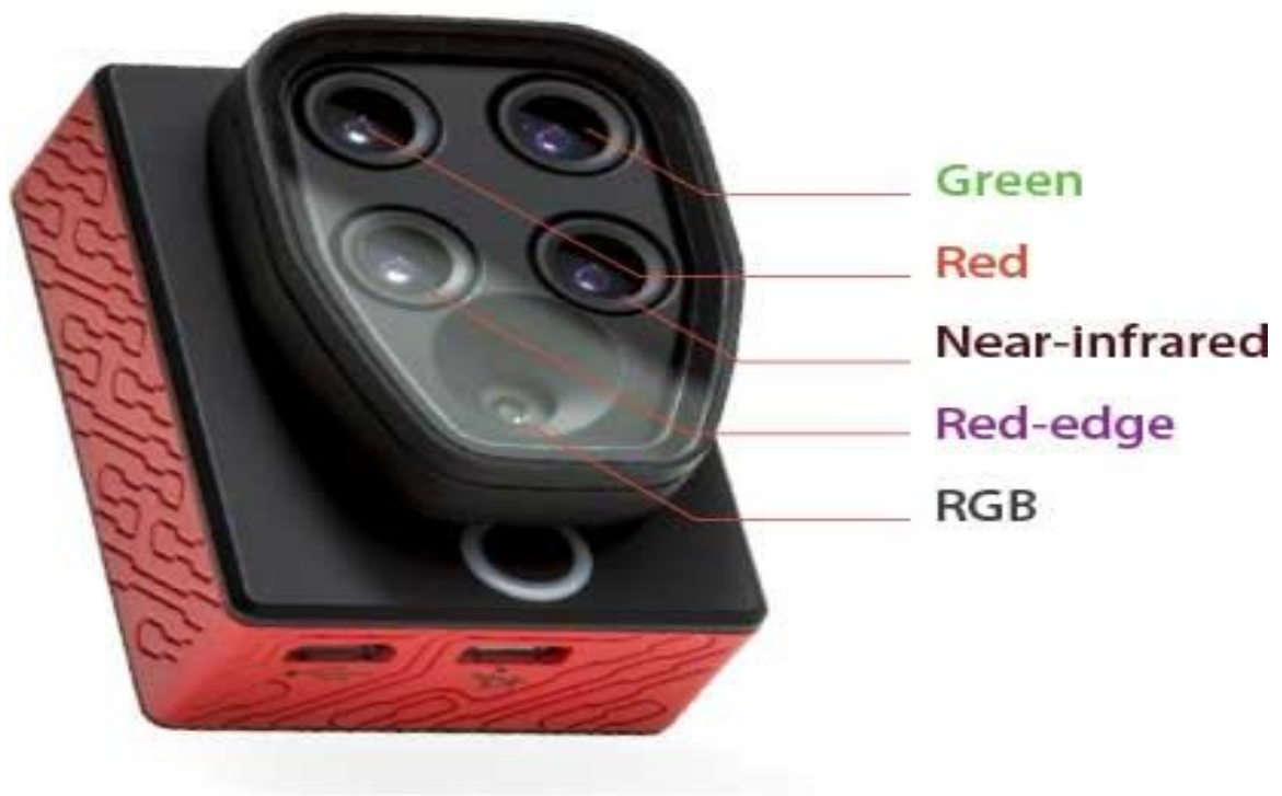
Figure 3. 3: Multispectral sequoia camera
