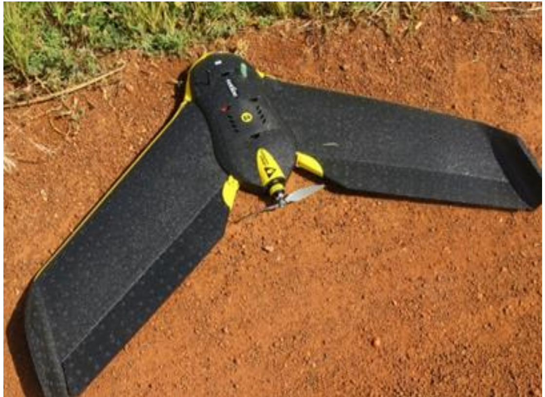
Figure 3. 2: The eBee fixed winged unmanned aerial vehicle
