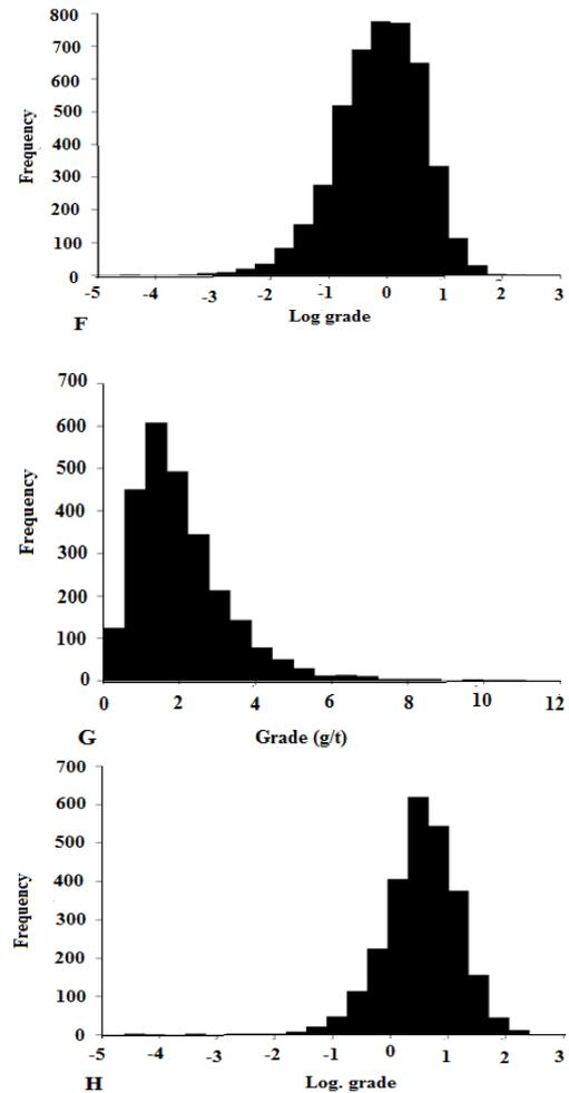
**Figure 8:** Plots of the histograms of the raw data and logarithms of grades for the separate reefs: (A) Frequency distributions of Au grades for A reef, (B) Logarithms of grade for A reef, (C) Frequency distributions of Au grades for CDE reef, (D) Logarithms of grade for CDE reef, (E) Frequency distributions of Au grades for F24 reef, (F) Logarithms of grade for CDE reef, (G) Frequency distributions of Au grades for G reef, (H) Logarithms of grade for G reef
