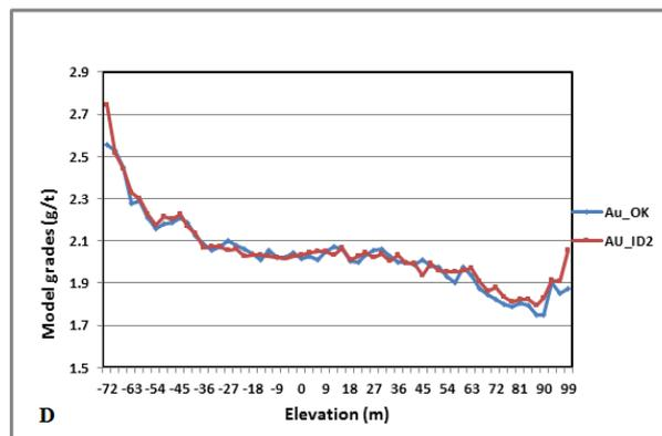
Figure 13: Comparison of estimated grades: (A) OK, ID, ID<sup>2</sup>, ID<sup>3</sup>, and ID<sup>4</sup> model for A reef, (B) OK, ID, ID<sup>2</sup>, ID<sup>3</sup>, and ID<sup>4</sup> model for CDE reef, (C) OK and ID<sup>2</sup> model for A reef, (D) OK, and ID<sup>2</sup> model for CDE reef.
