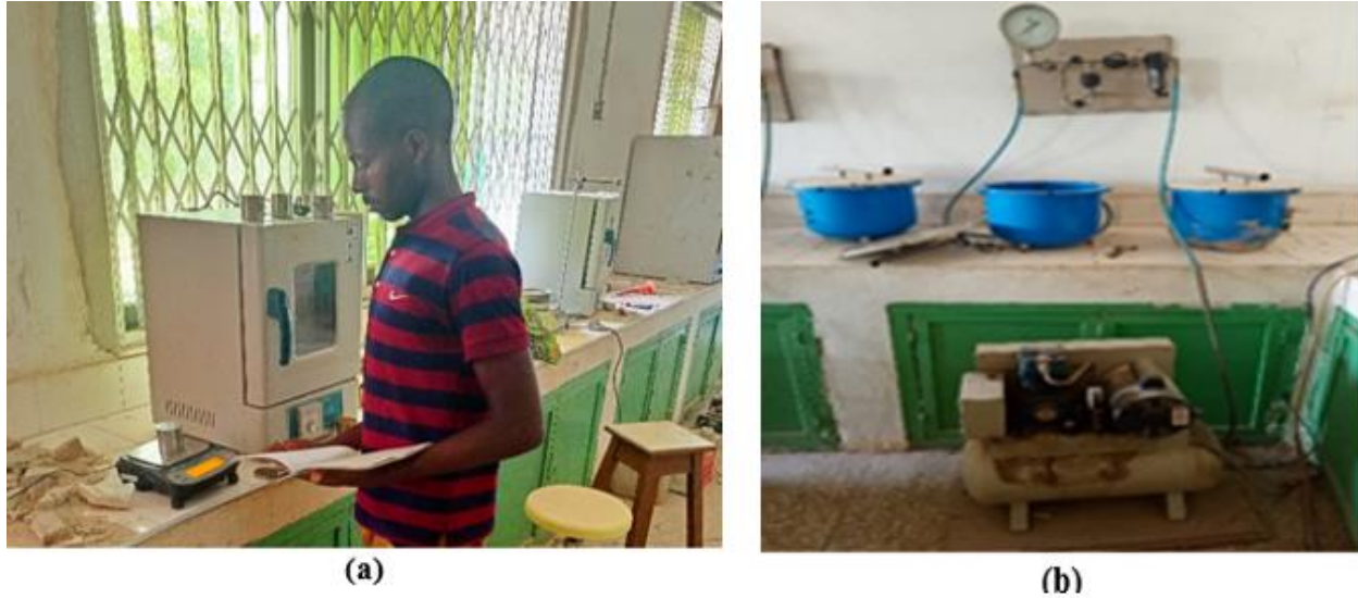
Figure 3.4: (a) Results of Bulk density in Laboratory and (b) Pressure Plate Apparatus
