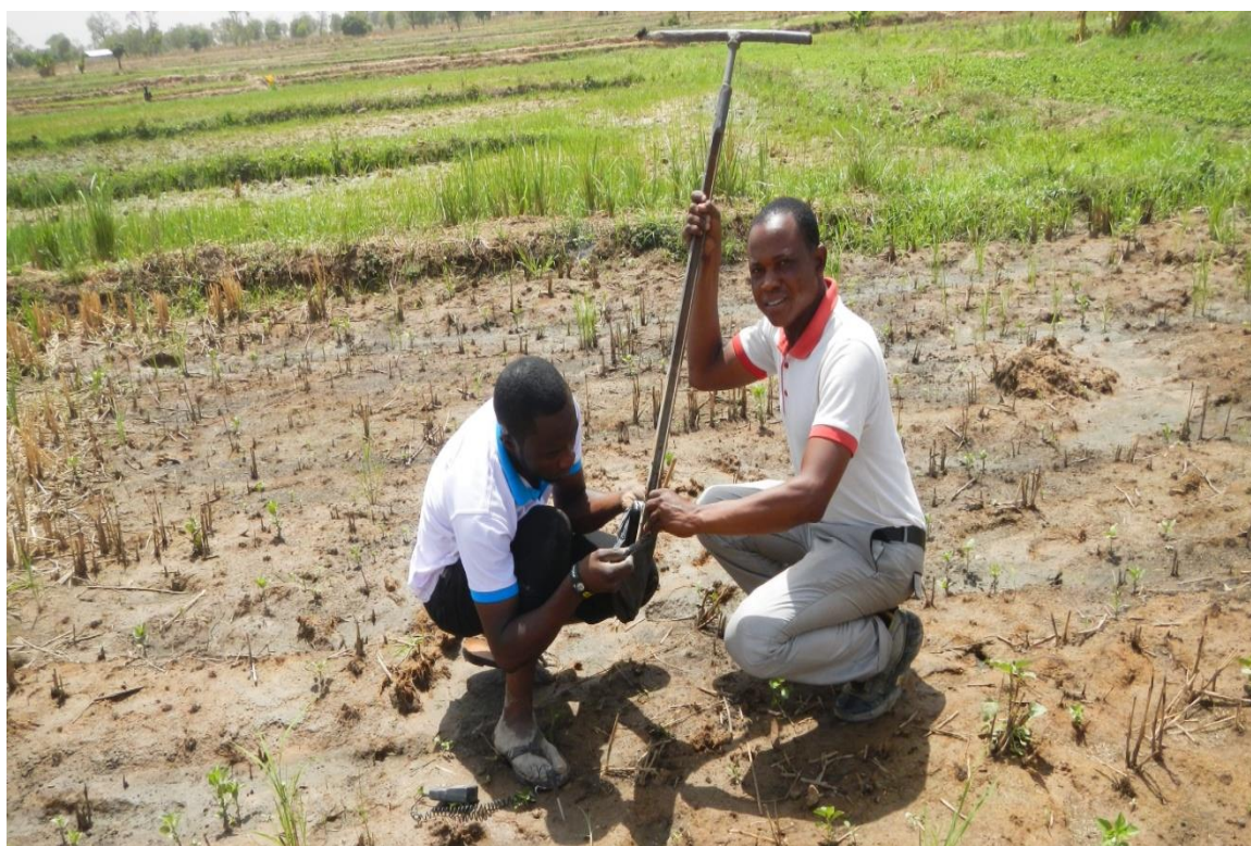
Plate 3.5: Field Soil Sampling Using Auger
