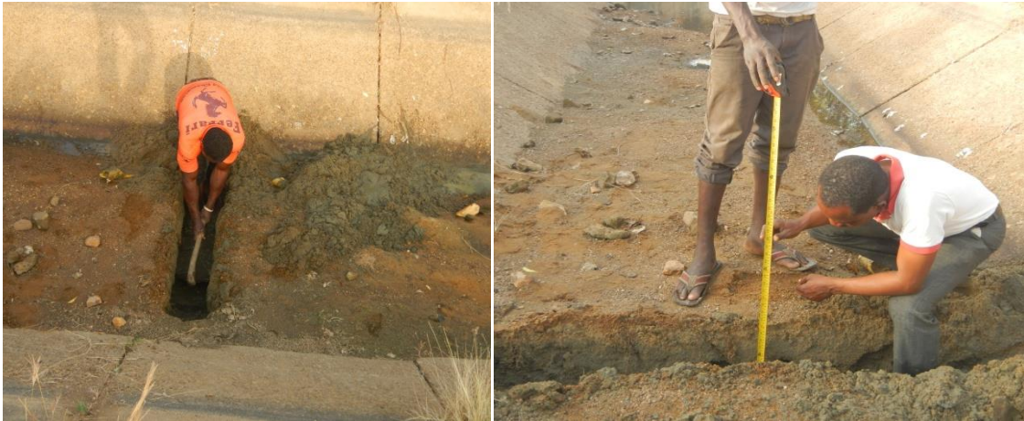
Plate 3.3: Profile Digging and Measurement of Depth of Sediments in a Main Canal
