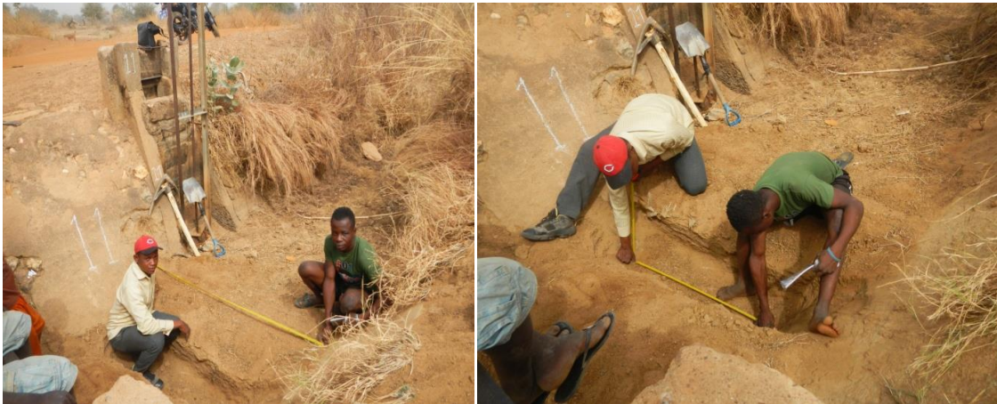
Plate 3.4: Measurement of Top Width in Contact with Sediments and Bottom Width in a Main Canal
