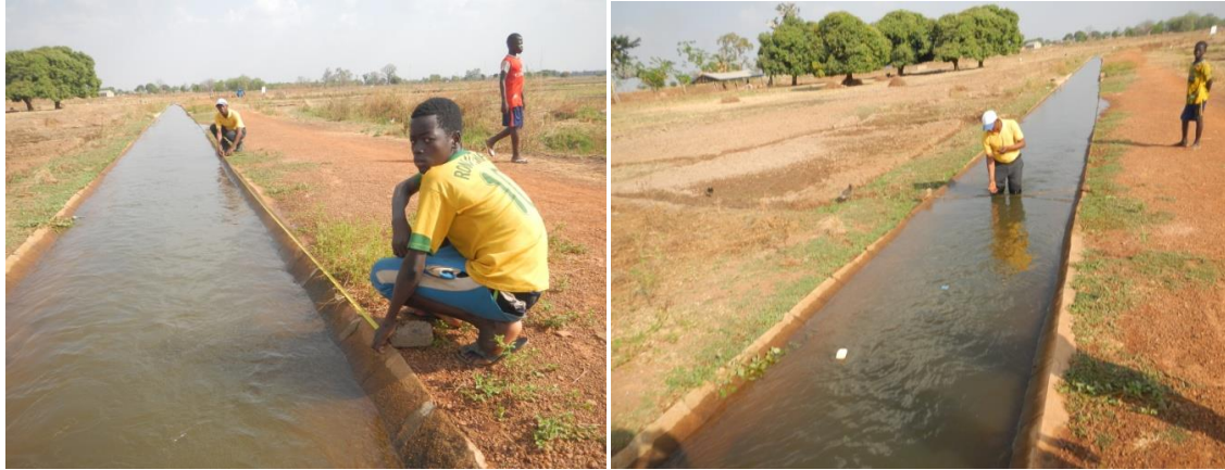
Plate 3.2: Measurement of Flow Velocity in Main Canal by Float Method
