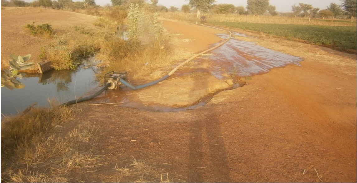
Plate 4.22: Lifting Water from Canal Using Water Pump in theVea Irrigation Scheme
