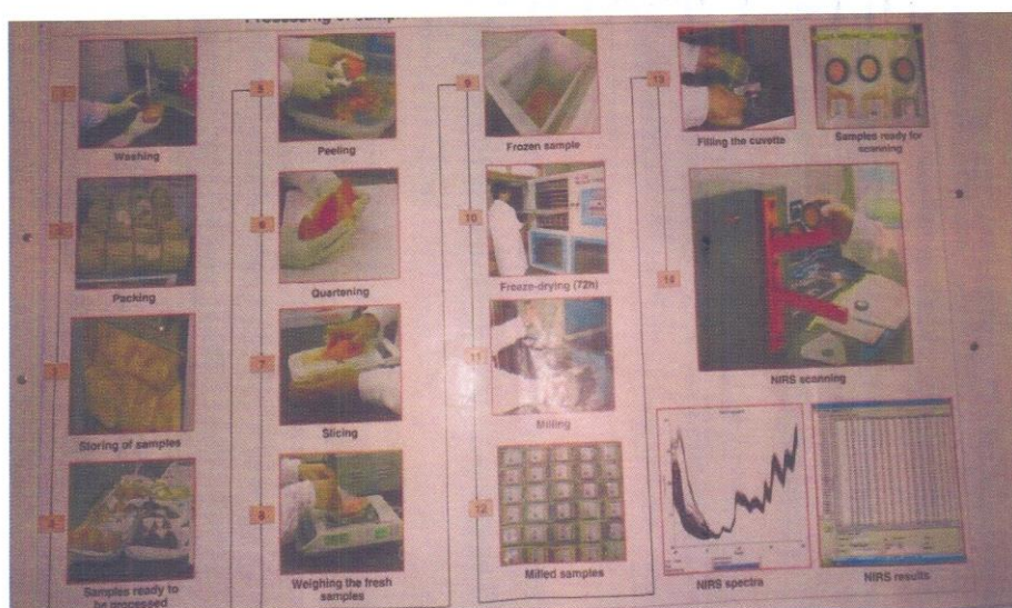
Plates 13: Summary of how roots were processed and analyzed at the sweetpotato laboratory
