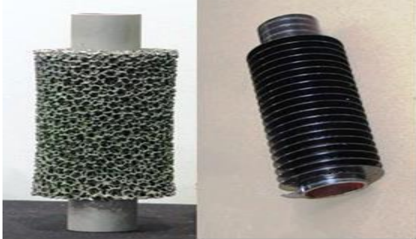
Figure 1. 9 Heat transfer application of metal foam (Bhaskar and Chaudhary 2016)
