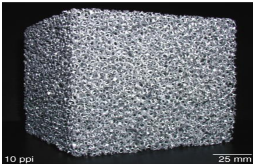
Figure 1. 10 A foam sample manufactured by sintering route (Bhaskar and Chaudhary 2016)
