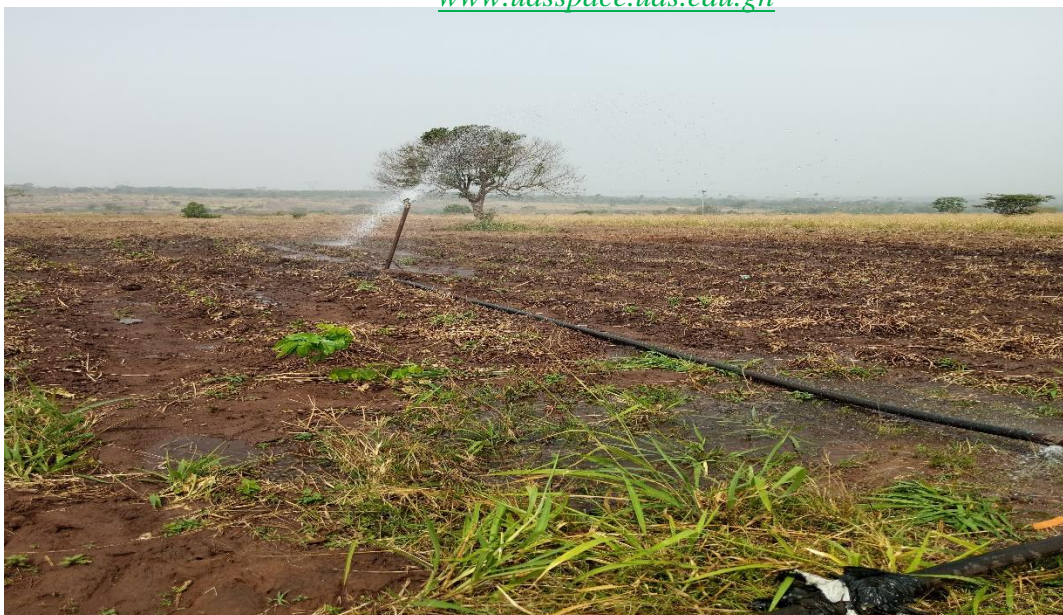
Figure 3.2: Water Distribution in the Field by the Rotating-impact Sprinkler
