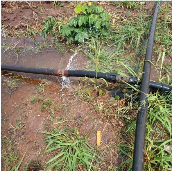
a) Leaking Pipe lateral with Unfit Coupling
