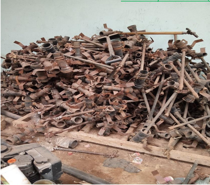
d) Faulty Sprinklers Deposited at the Scheme's Warehouse
