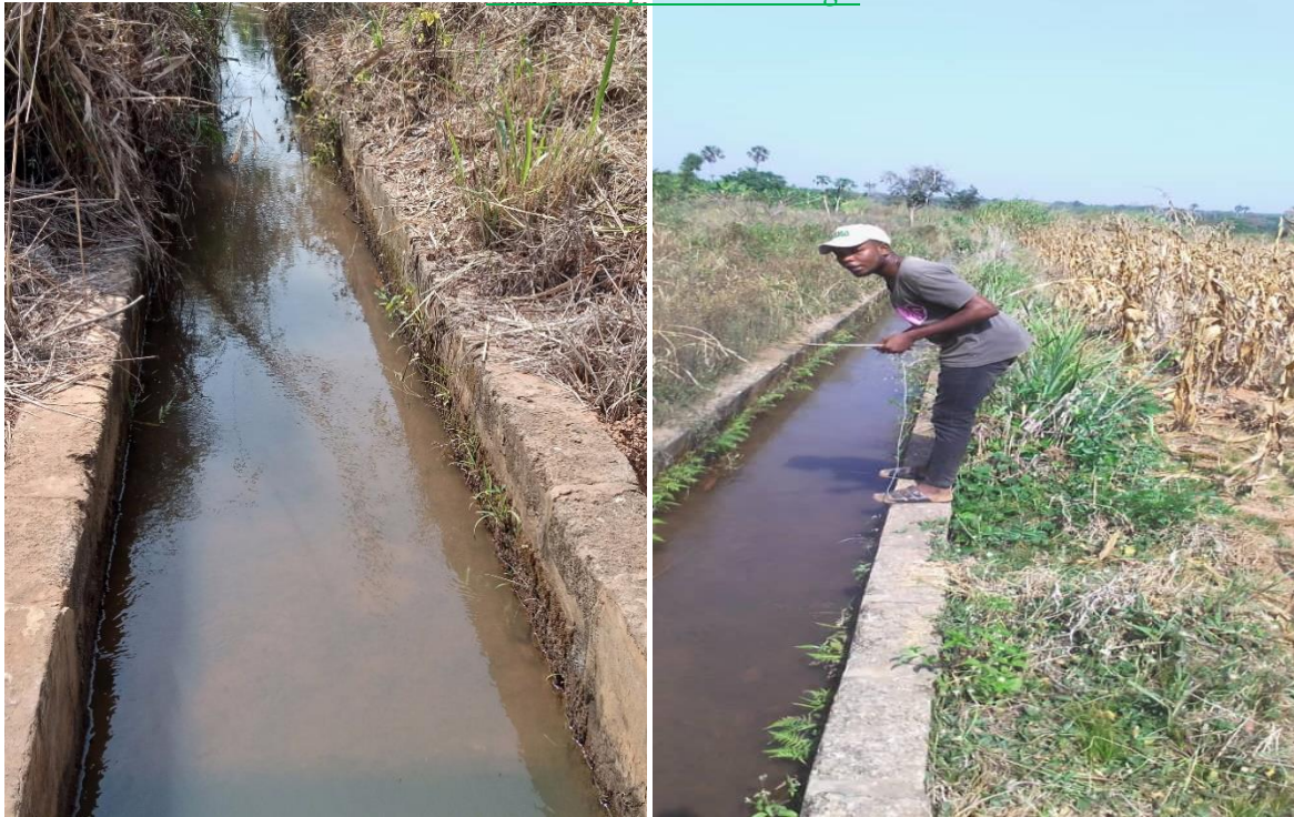
Plate 3.1: Measurement of Canal Dimensions and Flow-depth at Kaniago Irrigation scheme
